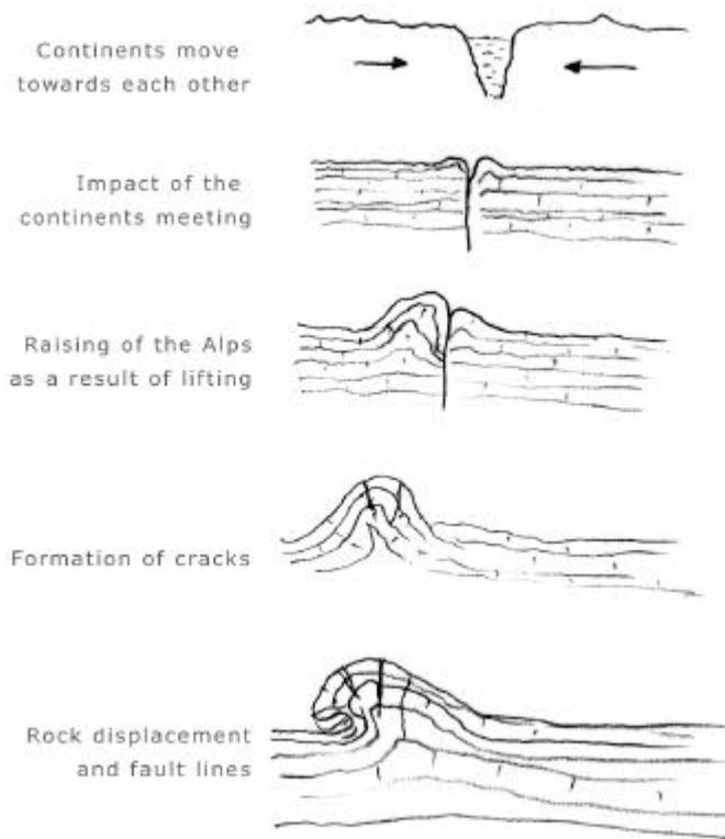
During a process of lifting the Alps were formed by rock masses arching up and the resultant tectonic cracks caused the formation of hollow areas in the mountains. Consequently outside influences, especially water, were able to play their part in the formation of the subterranean passages.
