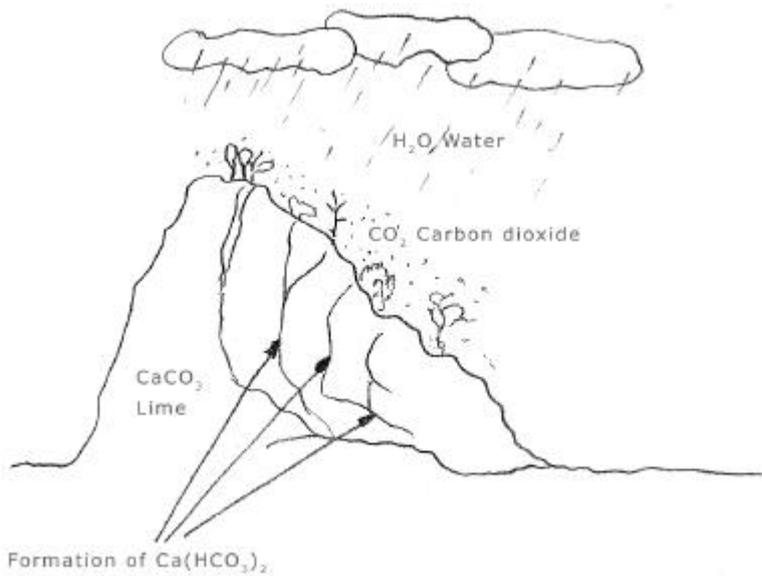
Corrosion is the chemical dissolving of rock (Lime CaCO<sub>3</sub>) by carbon dioxide (CO<sub>2</sub>) und water (H<sub>2</sub>O). Pure water has less H<sup>+</sup> ions and would not cause lime to dissolve. The introduction of CO<sub>2</sub> from the air and vegetation causes the formation of an aggressive acid :
